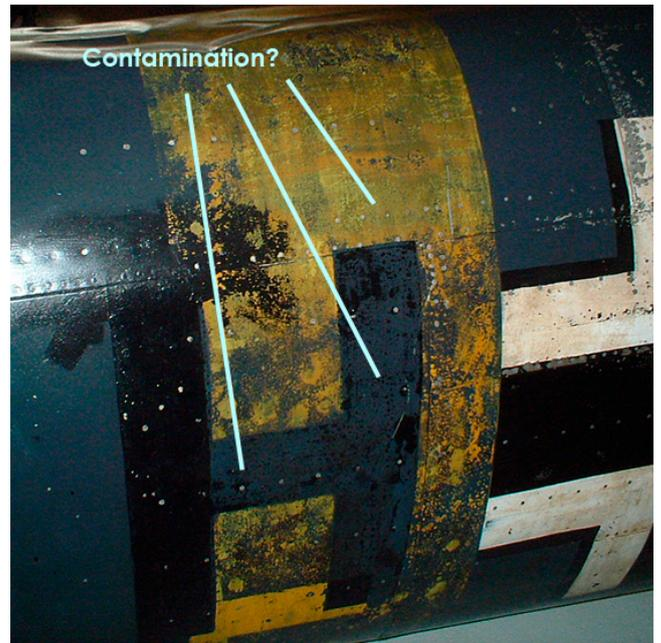
The over-exposed photography also revealed that 2398 had been *very considerably* re-painted during its operational lifetime. Evidence for such re-finishing is everywhere, but on the fuselage the various details of this work stand out all the better under flash exposure. This image, for example, shows re-painting around the code letters on the port side using a darker finish over the applique RLM 66, which might be the very dark grey colour identified above.
